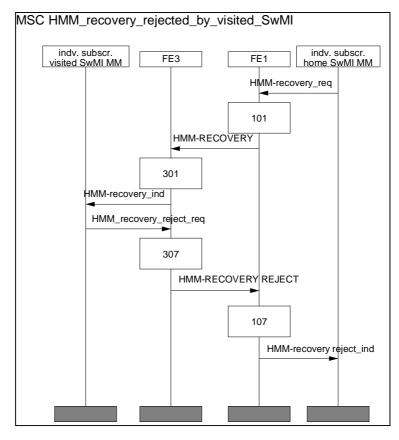
Figure 30.7: Rejection of HMM recovery
