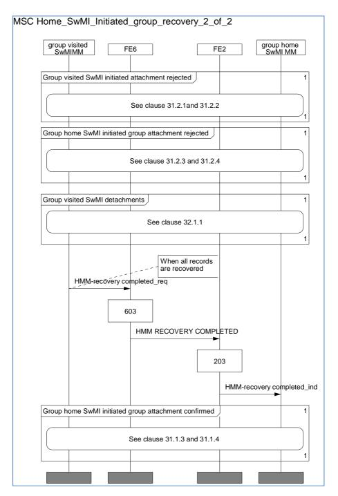
NOTE: Upon completion of the HMM recovery completed\_ind, the group home SwMI MM may invoke the group home SwMI MM initiated group attachment services for each group attachment that is recorded as valid in the group visited SwMI MM but on which the virtual group attachment has not been invoked.
