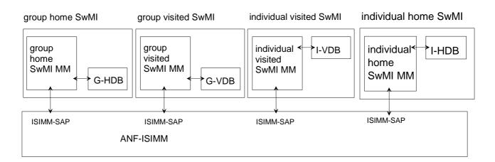
NOTE: The arrows illustrate the information exchange routes of the service. In the case of a solid arrow, the information exchange is mandatory; in the case of a broken arrow, the information exchange is conditinal. If the service is invoked against an individual subscriber the I-HDB and the I-VDB are involved; if against group the G-HDB and the G-VDB are involved.
