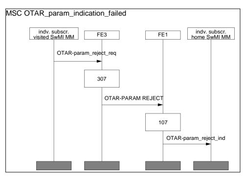
Figure 29.9: Failed subsequent use of OTAR SCK generation parameters
