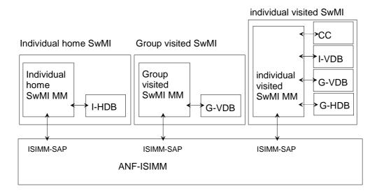
NOTE: The arrows illustrate the information exchange routes of the service. In the case of a solid arrow the information exchange is mandatory; in the case of a broken arrow the information exchange is conditional. The CC exists in the SwMI where the individual subscriber is now located (which might be the individual subscriber home SwMI or another individual subscriber visited SwMI) if the individual subscriber is engaged in a call when he migrates.
