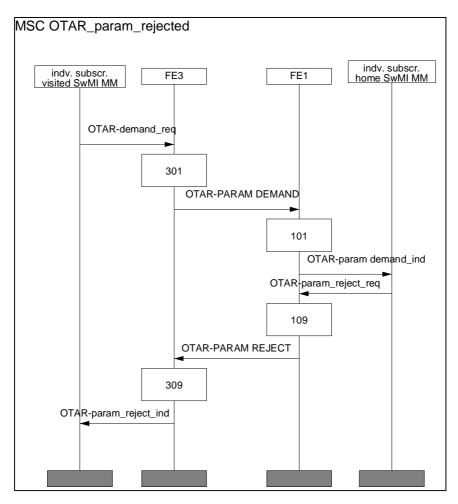
Figure 29.5: Failed OTAR parameter delivery
