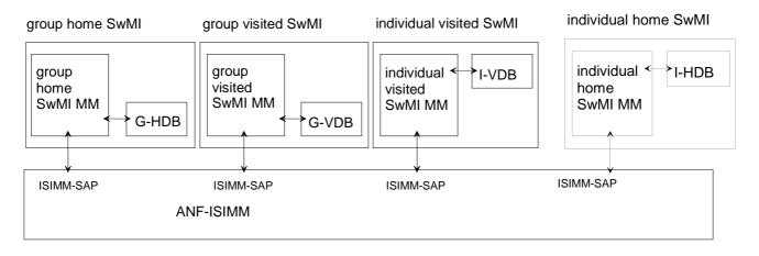
NOTE: The arrows illustrate the information exchange routes of the service. In the case of a solid arrow, the information exchange is mandatory; in the case of a broken arrow, the information exchange is conditional. If the service is invoked against an individual subscriber the I-HDB and the I-VDB are involved; if against group the G-HDB and the G-VDB are involved.
