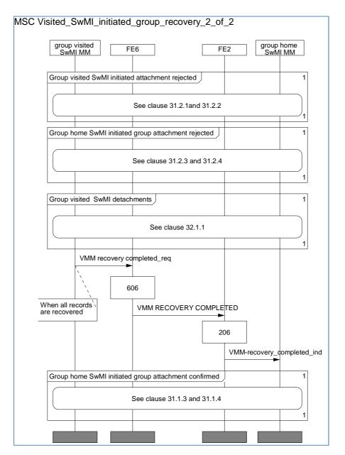
NOTE: Upon completion of the VMM recovery completed\_ind, the group home SwMI MM may invoke the group home SwMI MM initiated group attachment services for each group attachment that is recorded as valid in the group visited SwMI MM but on which the virtual group attachment has not been invoked.
